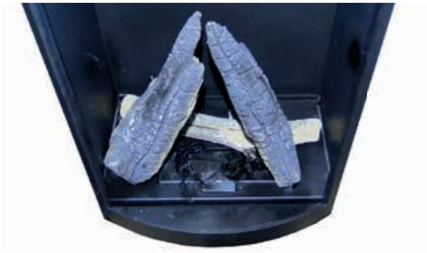
Place log 01 (R) on burner port BP 2. Pay attention that the log slides all the way over the burner port.
